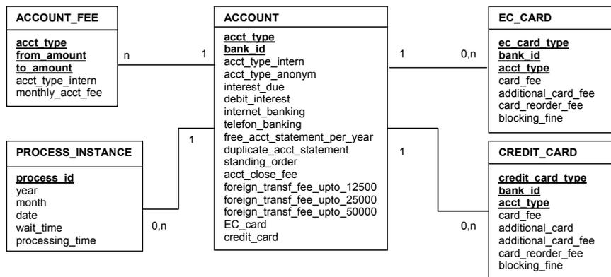
Figure 4: Data Model with Company Internal and External Data
