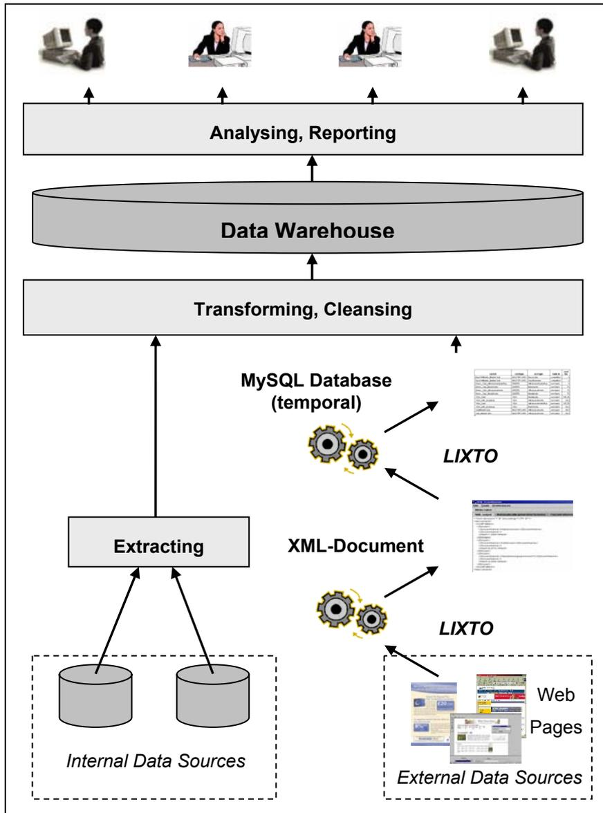
Figure 1: Architecture of the Online Bank's Data Warehouse
