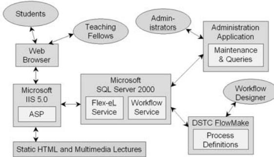
**Figure 1. Flex-eL Technology Architecture**
